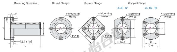
1 Body length is approximately 1.5 times of single type, and allowable moment is approximately 4 times. (See Allowable Load Comparison)
